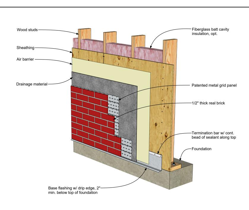
MCS Exterior Wall, Wood Stud Backing | Base of Wall Detail 03.02.01 Rev. 01/26/19
