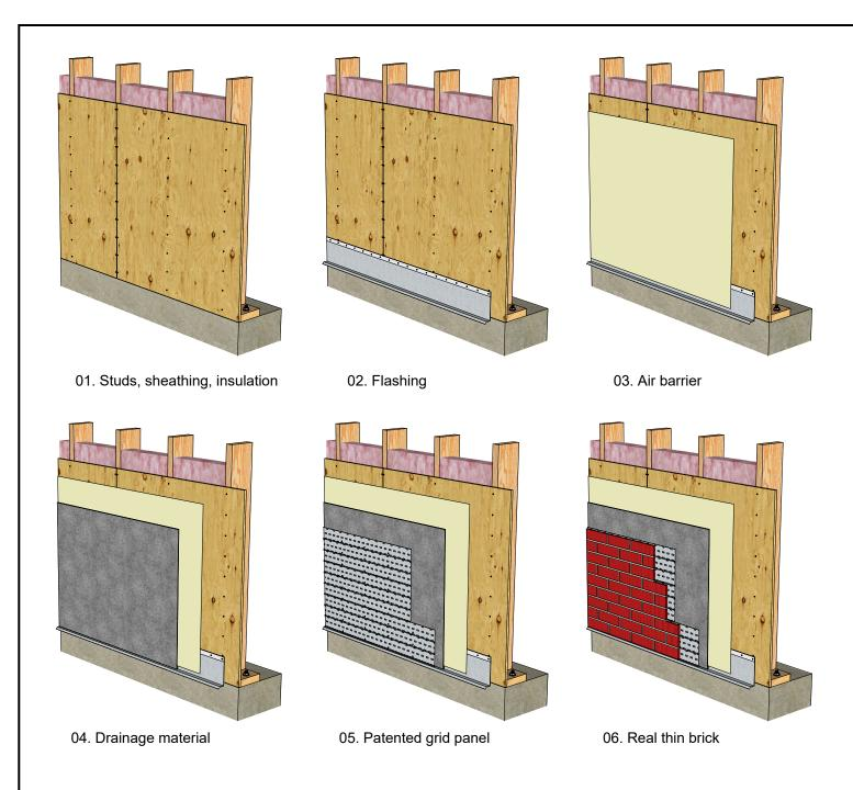
MCS Exterior Wall, Wood Stud Backing | Base of Wall Sequencing Detail 03.02.01 Rev. 01/26/19
