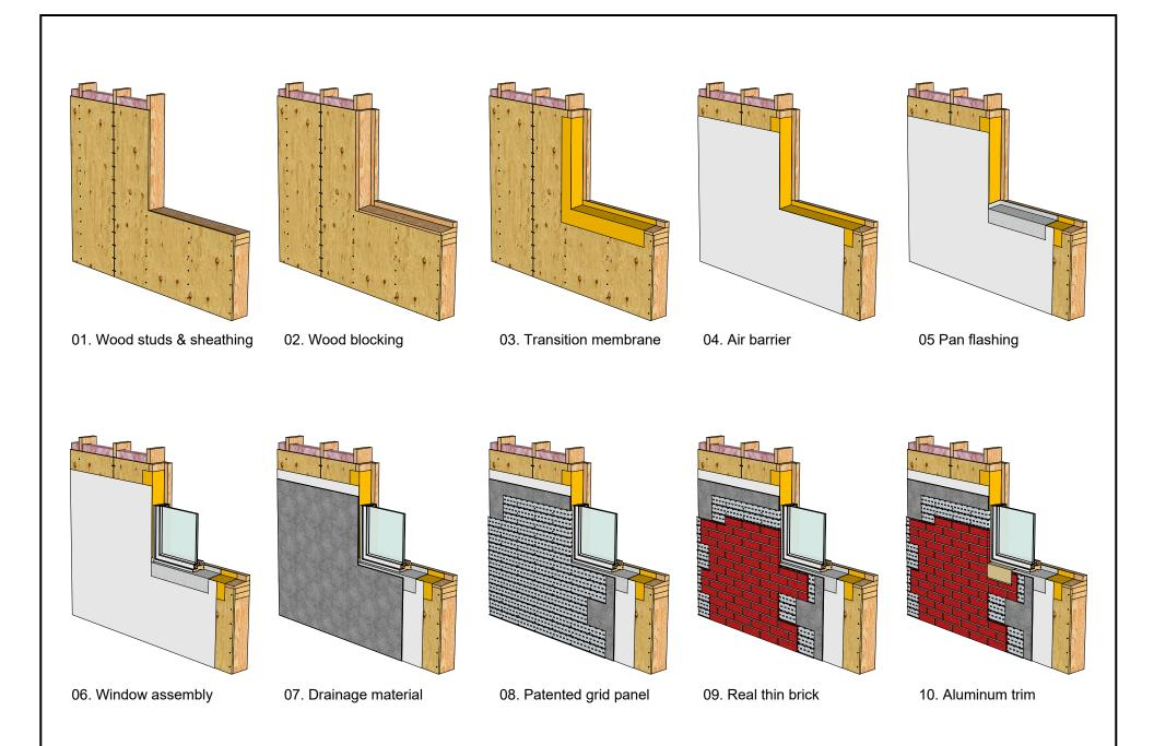
MCS Exterior Wall, CMU Backing | Window Sill Sequencing
