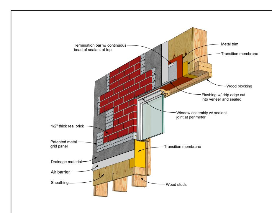
MCS Exterior Wall, Wood Stud Backing | Window Head Detail 03.02.03 Rev. 02/10/19
