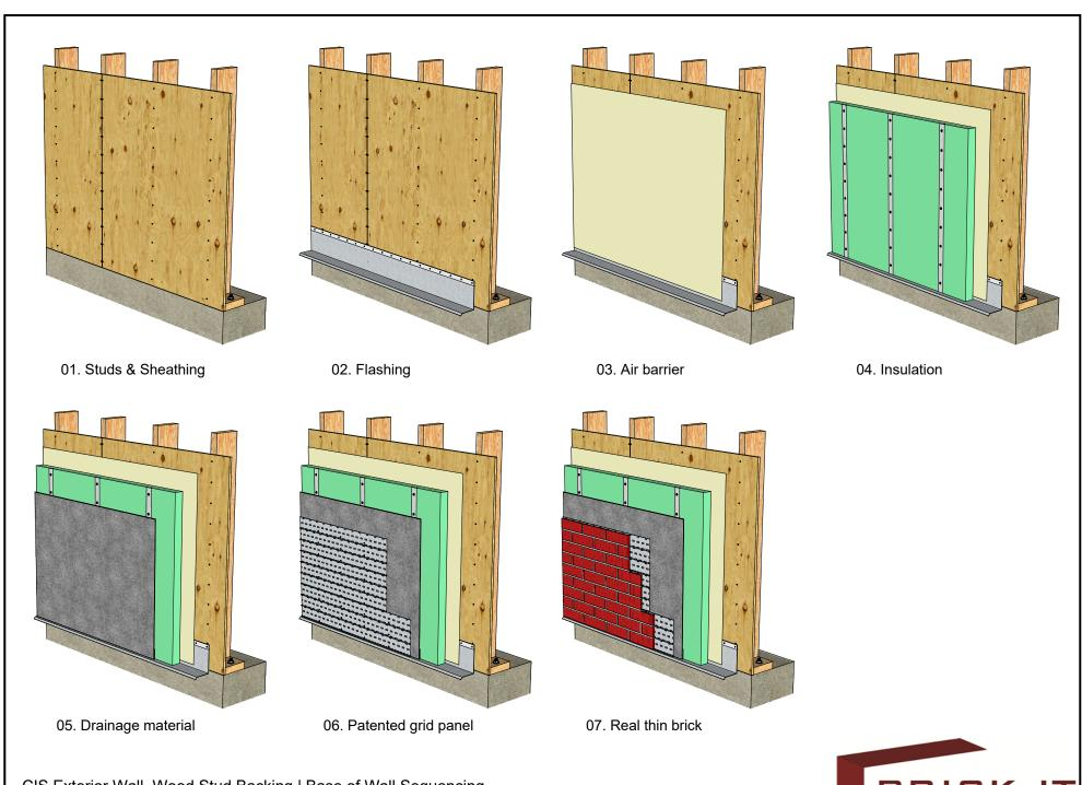
CIS Exterior Wall, Wood Stud Backing | Base of Wall Sequencing
