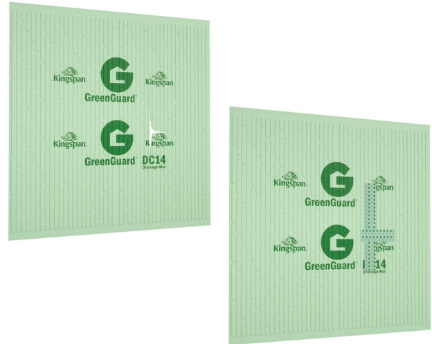
Figure 9: Repair of Small Damaged Area
