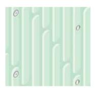
**Figure 1:**Proper Location of Fasteners
