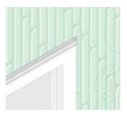
Figure 2: Installation of Drip Cap
