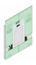
Figure 3: Installation of Upper Course of Kingspan GreenGuard® DC14 Drainage Mat
