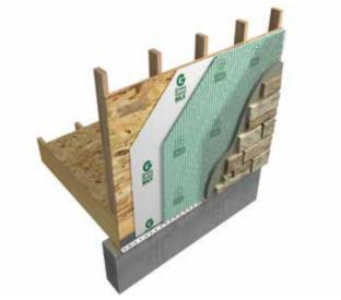
**Figure 7:** Finished Wall System-Adhered Stone Veneer
